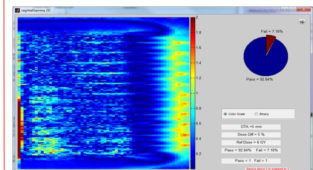
**Figure 3.** Sagittal film Gamma analysis for Trial 3 with a 5%/5mm passing criteria.
