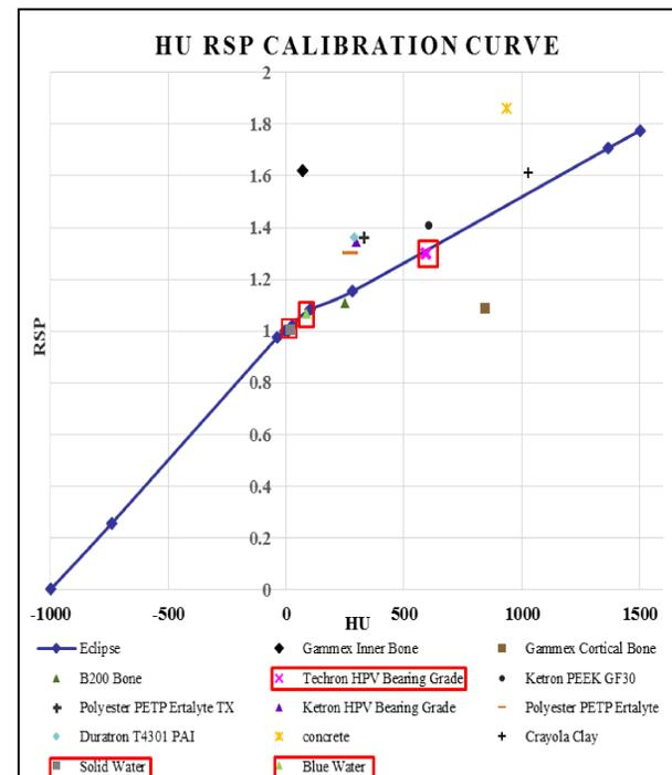
**Figure 2.** Relative Stopping Power (RSP) versus Hounsfield unit calibration curve comparing tested materials with Eclipse treatment planning system. The selected phantom materials are highlighted.
